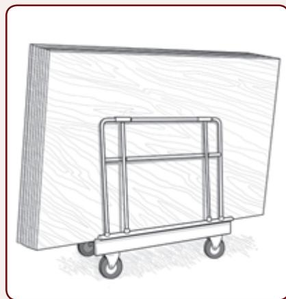
Drywall dolly keeps materials off ground & moves sheet materials on floors.
