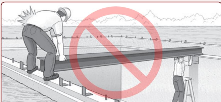
Placing a steel I-beam by hand across foundation wall can result in a disabling injury or death.
