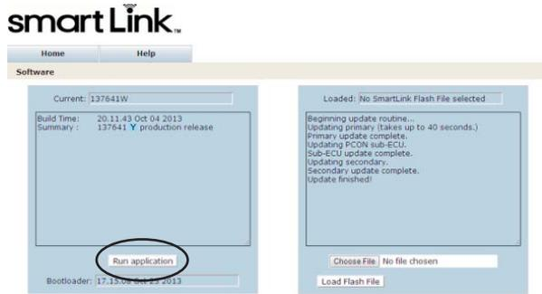
Note: Verify that the firmware number is displayed in the box marked "**Current:**". Firmware number 137641Y (rev Y or above).
